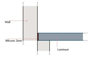
Use plastic film or adhesive rubber tape to protect the adjacent surface when applying the silicone. If the top consists of several sections, care should be taken when positioning them to avoid knocking the exposed edges. This operation can be facilitated by inserting spacers, to be removed once the slabs are in place. Join the two sections using silicone products, or clear or coloured adhesives, taking care to remove any residue after application.
