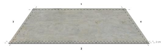
Cuts to loosen a 12 mm or 20 mm slab.
