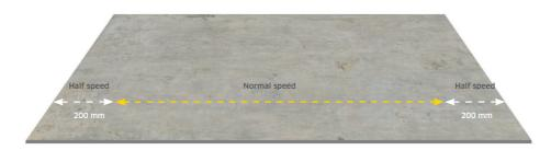
These recommendations only apply to 12 mm and 20 mm slabs. Any other thickness can be cut without having to take these steps into account.
