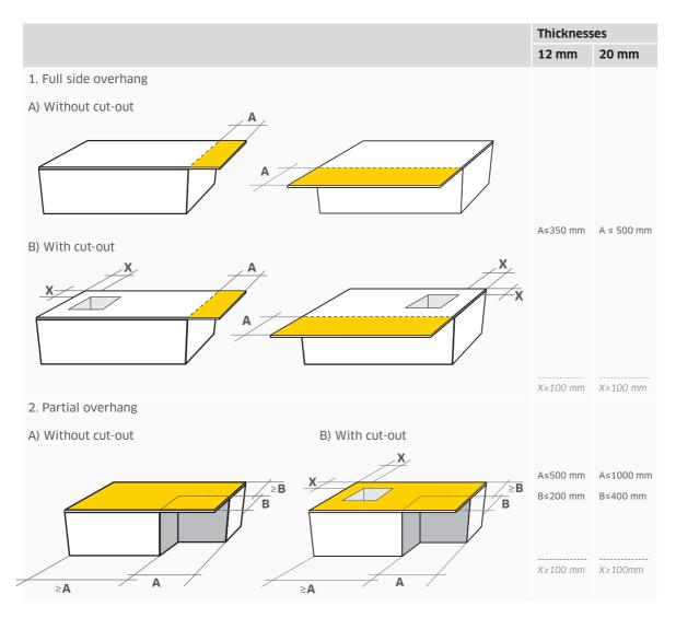
Occasional maximum static load = 100 kg It is recommendable to reinforce the  $\boldsymbol{X}$  sections with additional reinforcements of expanded polyurethane.
