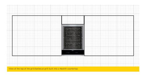
$\cdot$  Leaving a minimum space of 5 mm between the grill/barbecue grill and filling with thermal insulation such as fiberglass thermal insulation tape is recommended.
