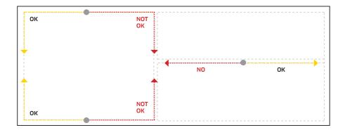
First cutting towards the edge of the slab from the hole or in parallel to the edge of the slab and following this direction to finish the part is recommended. Making the first cut towards the center of the slab is not recommended.
