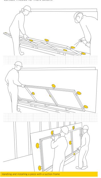
If this type of frame is not available, an aluminum rod or similar element, secured with several jacks, can also be used.
