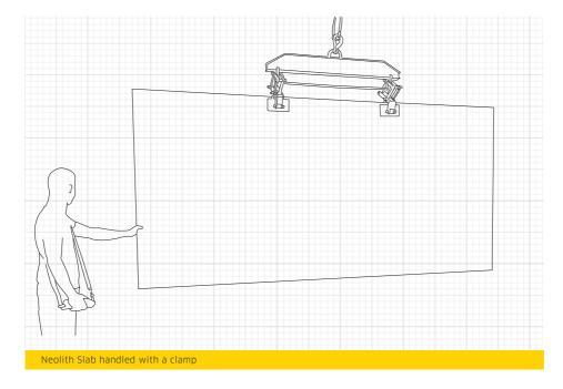
The additional width of this clamp will prevent the slab from bending during handling to, thus, prevent undesirable breakage.
