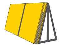
The supports must be able to hold the entire surface of the part during transport. Supports that are too small may cause the part to break:
