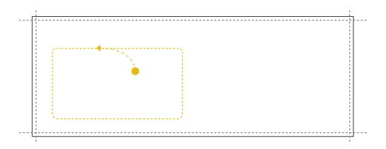
First drill a hole inside the cutout, using the crown bit. Afterwards, use the router bit to get closer to the cutting line.
