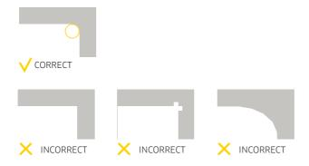
The correct way to create a cutout, except with waterjet and digital control bits, is to first drill the corners and then the rest of the cuts.
