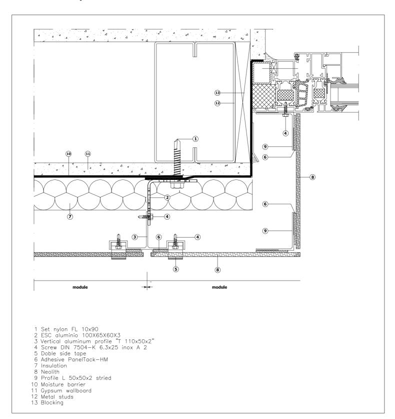
Dintel detail. Strongfix system. Vertical section
