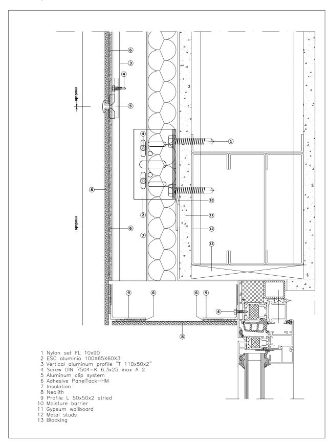
Sill detail. Strongfix system. Vertical section
